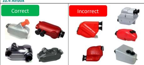
Airbox examples, intakes can be: front side or top
